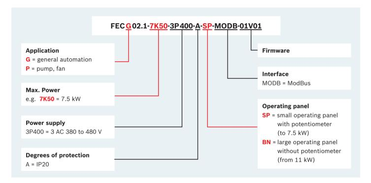
Frequency Converter Fe is available in two variants to ensure optimal integration:
